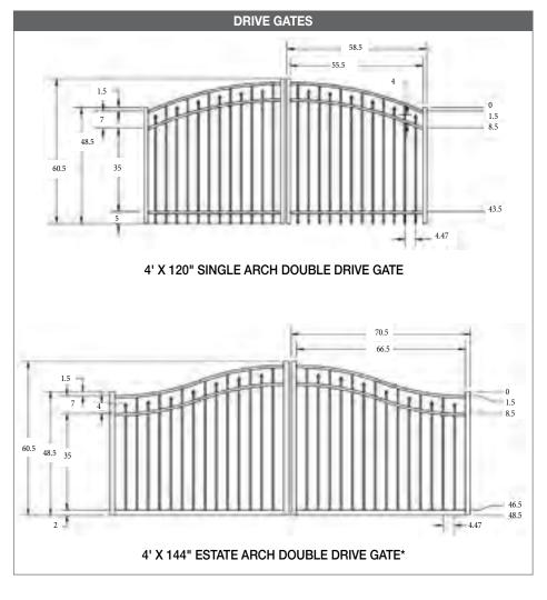
stability, all gates beyond 6' wide are built with a thicker bottom frame that creates a flush bottom finish.
