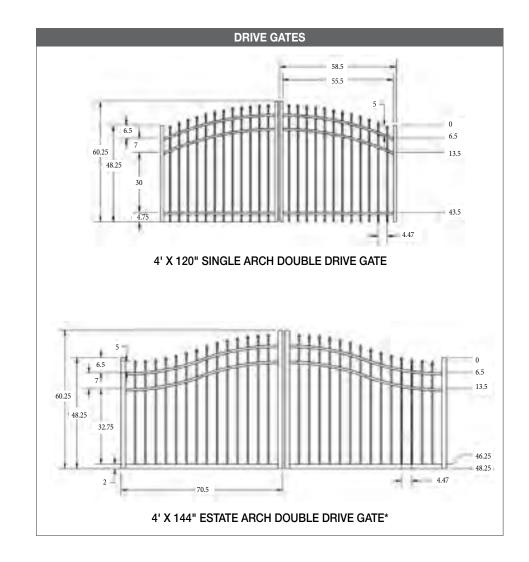
\*PLEASE NOTE: For additional strength and stability, all gates beyond 6' wide are built with a thicker bottom frame that creates a flush bottom finish.
