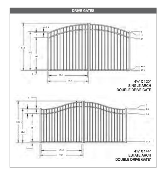
\*PLEASE NOTE: For additional strength and stability, all gates beyond 6' wide are built with a thicker bottom frame that creates a flush bottom finish.
