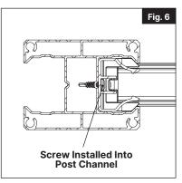
From the hardware kit, use one (1) #10 x 3/4" screw and attach to post near the center (Fig. 6).
