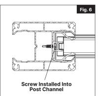
Install wood infill boards into the post channel and into the bottom rail channel. Repeat for remaining boards (Fig. 7).
