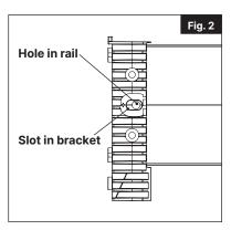
Align the pre-drilled holes on the rail with the slot in the bracket (Fig. 2).
