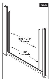
Insert the 62" PVC post channels from the infill kit into posts (Fig. 5). The bottom of the channel should sit on top of the bottom rail bracket.
