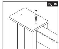
Install post trim cover. Insert fastener clip into opposite sides on trim cover. Slide two halves around base of post.
